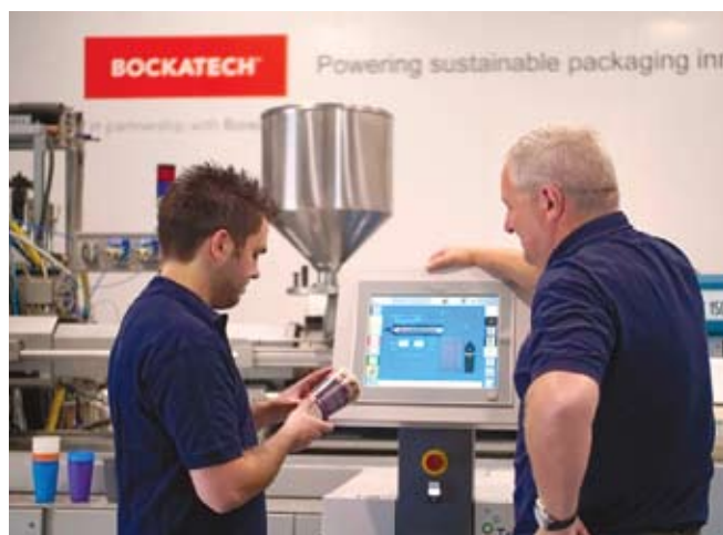
Specialists at the Bockatech R&D Centre with a Trexel MuCell P-300 Nitrogen delivery system (picture: Bockatech)
