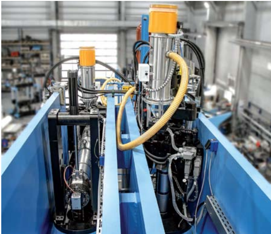
Two injection units are mounted separately on the top of the clamping frame modules and are thus easily accessible
