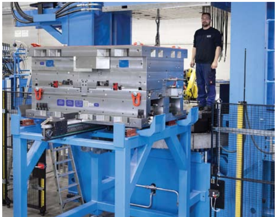
Tool changing station which, can be docked to the machine using an indoor crane
