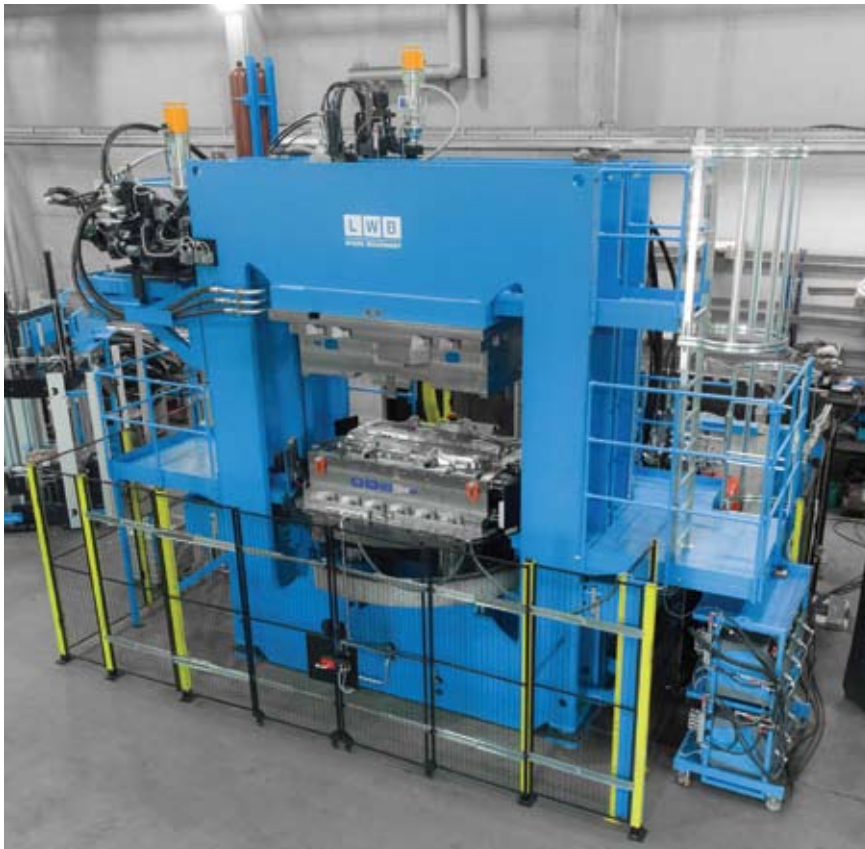
The alternative machine concept from LWB-Steinl, derived from the VR-vertical-machine-series with modular frame-shaped clamping unit and a horizontal orientated turntable, supported by four pressure units (Pictures: LWB-Steinl, ELDISY)
